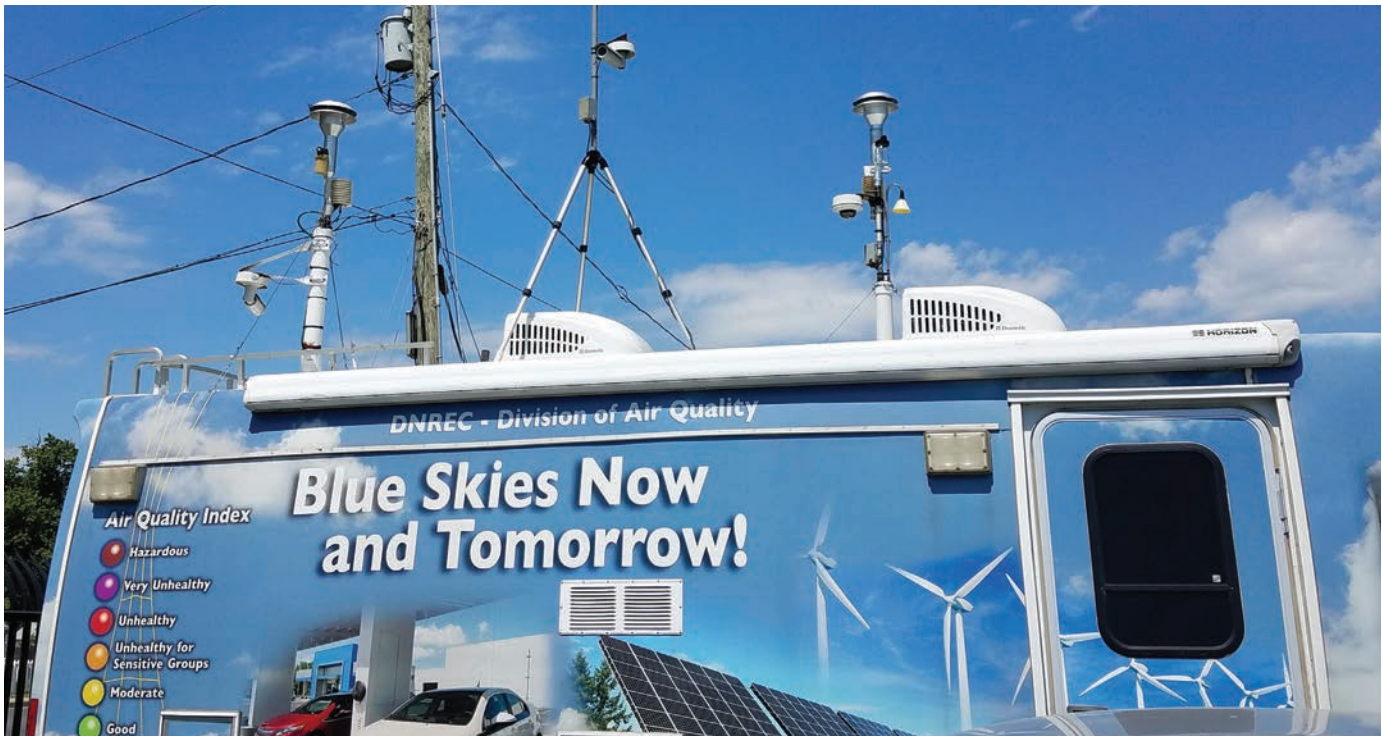
Mobile air monitoring stations like this one from the Delaware Department of Natural Resources and Environmental Control can allow communities to obtain air pollution data from locations without permanent monitoring but where pollutant levels may be high.
